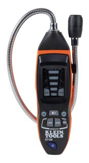
The ET120 is an easy-to-use tester that provides audible and visual alarms in the presence of methane, propane and other combustible gases at concentrations as low as 50 ppm, making it the perfect choice for HVAC professionals.
